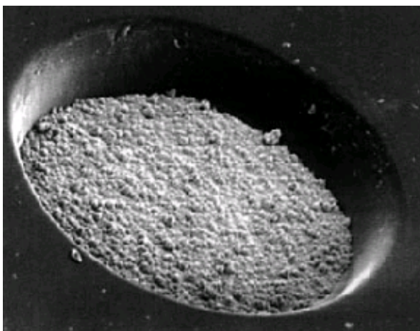
Figure 2. A laser drilled via in polyimide dielectric
