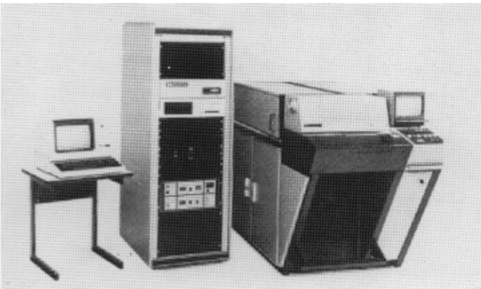
Figure 21 Laser trimmer for thickfilm hybrid circuits, ESI Model 44
