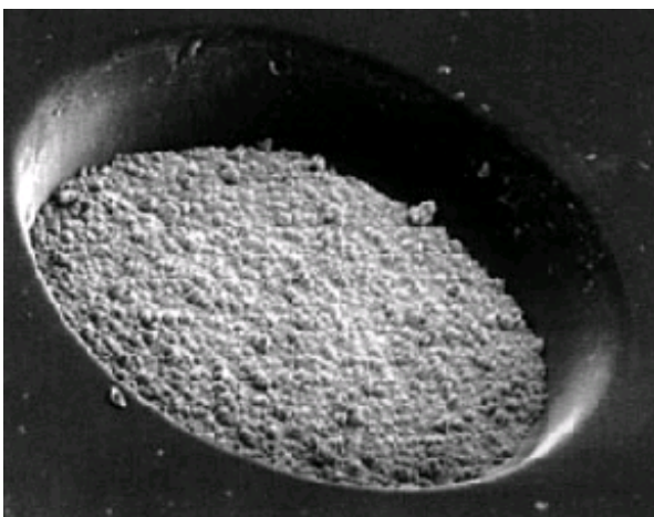
Figure 2. A laser drilled via in polyimide dielectric
