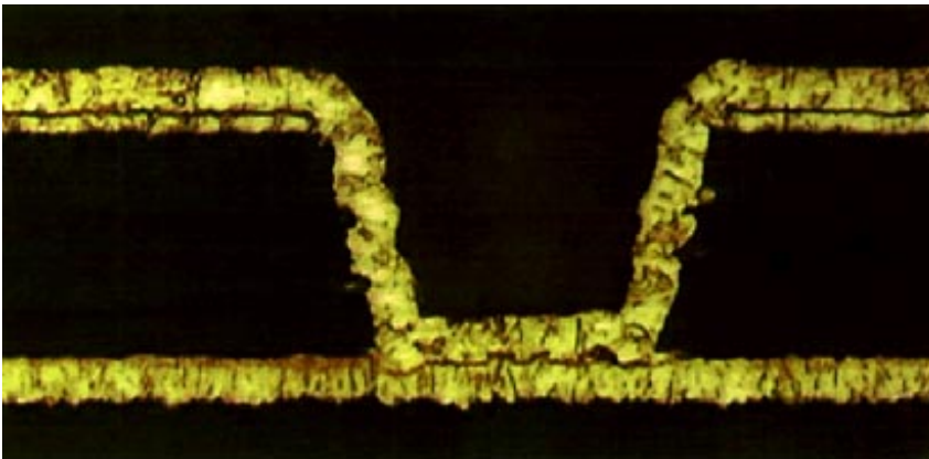
Figure 3: Cross-section of metalised laser-drilled via
