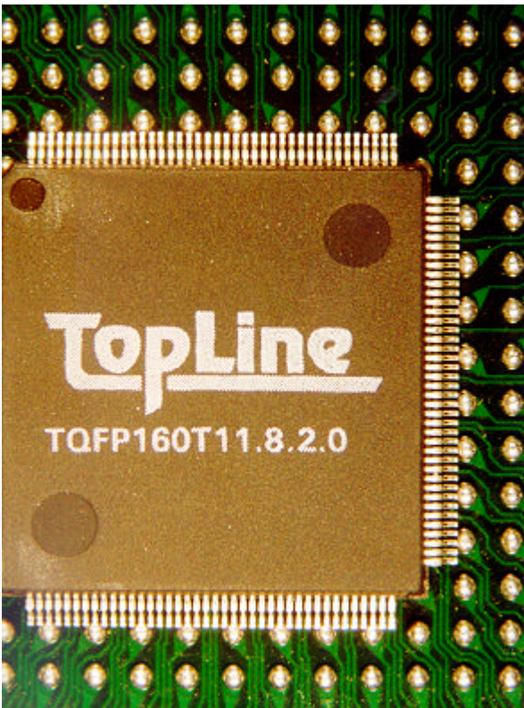
Figure 2. A 160-lead 0.3 mm (11.8 mil) pitch QFP placed on a grid of 1.5 mm pitch spheres (bottom side of a PBGA S225).
