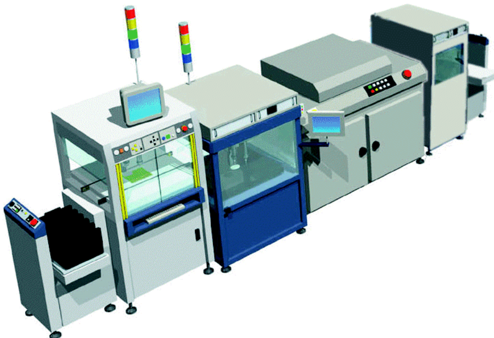
Figure B11. Flip-chip assembly line containing a separate flux dispensing unit. (Photo courtesy of Asymtek.)
